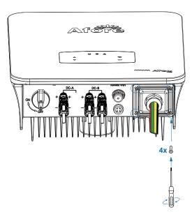
Fix the junction box with the wiring cover screws in the accessories, and tighten the waterproof connector.
