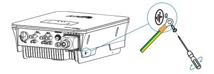
Fix the yellow-green PE wire to the ground hole on the lower right side of the inverter with screws, make sure that the PE terminal is properly grounded.
