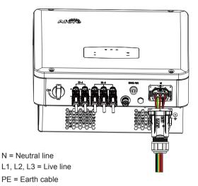
Use the hexagon wrench to loosen the screws in the terminal to a certain distance, insert the wire beam into N, L1, L2, L3, PE hole position and use a hexagon wrench to tighten the screw.
