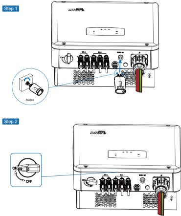
Turn on the DC switch and AC circuit breaker, and wait until the LED indicator on the monitoring module flashes, indicating that the monitoring module is successfully connected.
