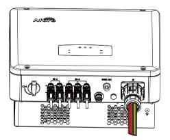
Insert the wiring box into the AC interface and check whether the insertion is in place.
