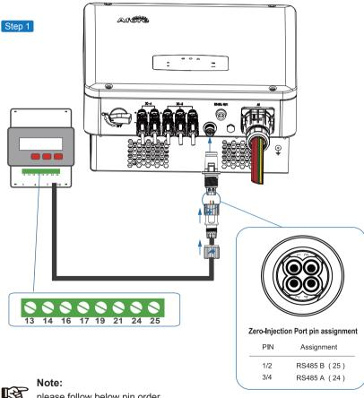
please follow below pin order RS485B (Pin 1/2) to three-phase meter (Pin 25) RS485A (Pin 3/4) to three-phase meter (Pin 24)
